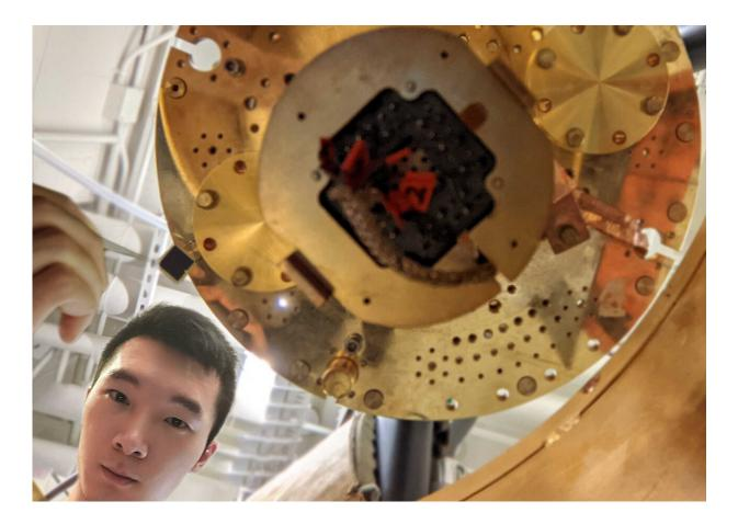
Zhiren (Isaac) Zheng holds up a sample of the new ferroelectric structure created by MIT researchers and colleagues (small black square with gold edges above Zheng's head). The gold structure is the inside of a Cryogen Free Dilution Refrigerator that the researchers used to measure the new ferroelectric structures. Credit: Sergio de la Barrera, MIT
