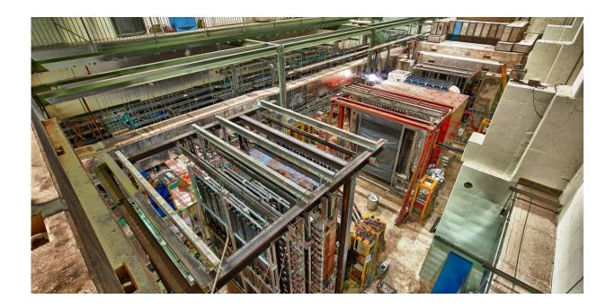
The apparatus used in the experiment. The proton beams pass through each of the shown layers. Credit: Fermi National Accelerator Laboratory
