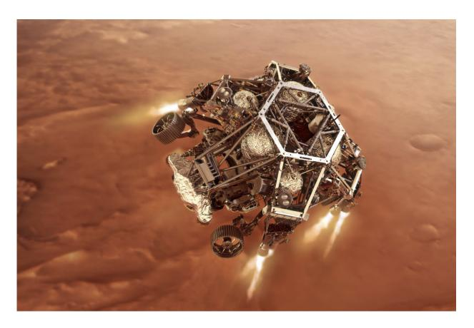
In this illustration provided by NASA, the Perseverance rover fires up its descent stage engines as it nears the Martian surface.. This phase of its entry, descent and landing sequence, or EDL, is known as "powered descent." (NASA/JPL-Caltech via AP)
