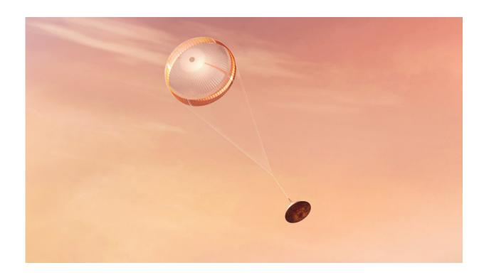
In this illustration made available by NASA, the Perseverance rover deploys a supersonic parachute from its aeroshell as it slows down before landing on the surface of Mars. (NASA/JPL-Caltech via AP)
