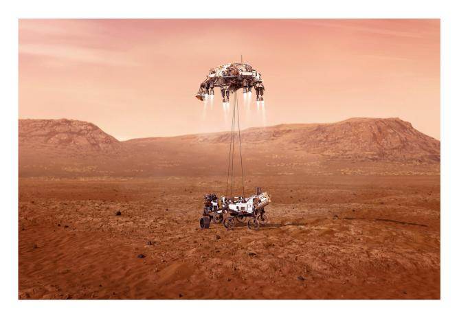
This illustration provided by NASA shows the Perseverance rover, bottom, landing on Mars. Hundreds of critical events must execute perfectly and exactly on time for the rover to land safely on Feb. 18, 2021. Entry, Descent, and Landing, or "EDL," begins when the spacecraft reaches the top of the Martian atmosphere, traveling nearly 12,500 mph (20,000 kph). EDL ends about seven minutes after atmospheric entry, with Perseverance stationary on the Martian surface. (NASA/JPL-Caltech via AP)
