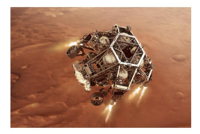
In this illustration provided by NASA, the Perseverance rover fires up its descent stage engines as it nears the Martian surface.. This phase of its entry, descent and landing sequence, or EDL, is known as "powered descent." (NASA/JPL-Caltech via AP)
