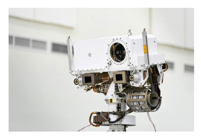
This July 23, 2019 photo made available by NASA shows the head of the Mars rover Perseverance's remote sensing mast which contains the SuperCam instrument in the large circular opening, two Mastcam-Z imagers in gray boxes, and next to those, the rover's two navigation cameras, at the Jet Propulsion Laboratory in Pasadena, Calif. The robotic vehicle will hunt for rocks containing biological signatures, if they exist. (NASA/JPL-Caltech via AP)
