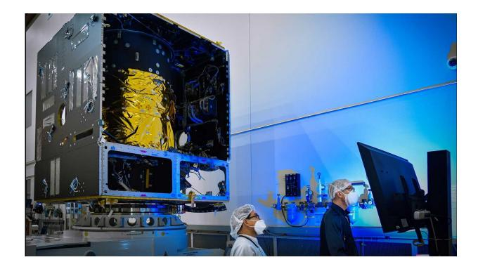
Technicians power on the main body of NASA's Psyche spacecraft, called the Solar Electric Propulsion (SEP) Chassis, at Maxar Technologies in Palo Alto, California, in November 2020. Credit: Maxar Technologies
