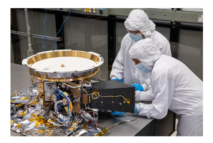
Two engineers work on L'Ralph, the most complicated instrument that will fly on the Lucy mission to Jupiter's Trojan asteroids. It is actually two instruments in one. The Multispectral Visible Imaging Camera (MVIC), will take visible light color images. The Linear Etalon Imaging Spectral Array (LEISA), will collect infrared spectra. Credit: NASA/Goddard/Barbara Lambert/Desiree Stover
