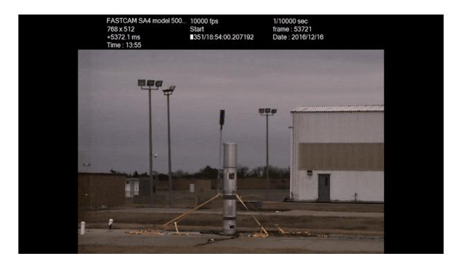
A ground test of the water canister release. Credit: NASA's Wallops Flight Facility
