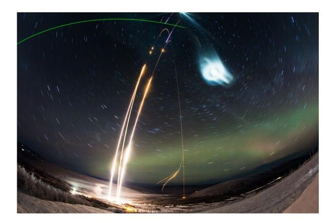
Time lapse of the Super Soaker launch. Three rockets launched with the mission, two using vapor tracers to track wind movement and one releasing a water canister to seed a polar mesospheric cloud. The green laser beam visible at the top left is the LIDAR beam used to measure the artificial cloud. Credit: NASA's Wallops Flight Facility/Poker Flat Research Range/Zayn Roohi
