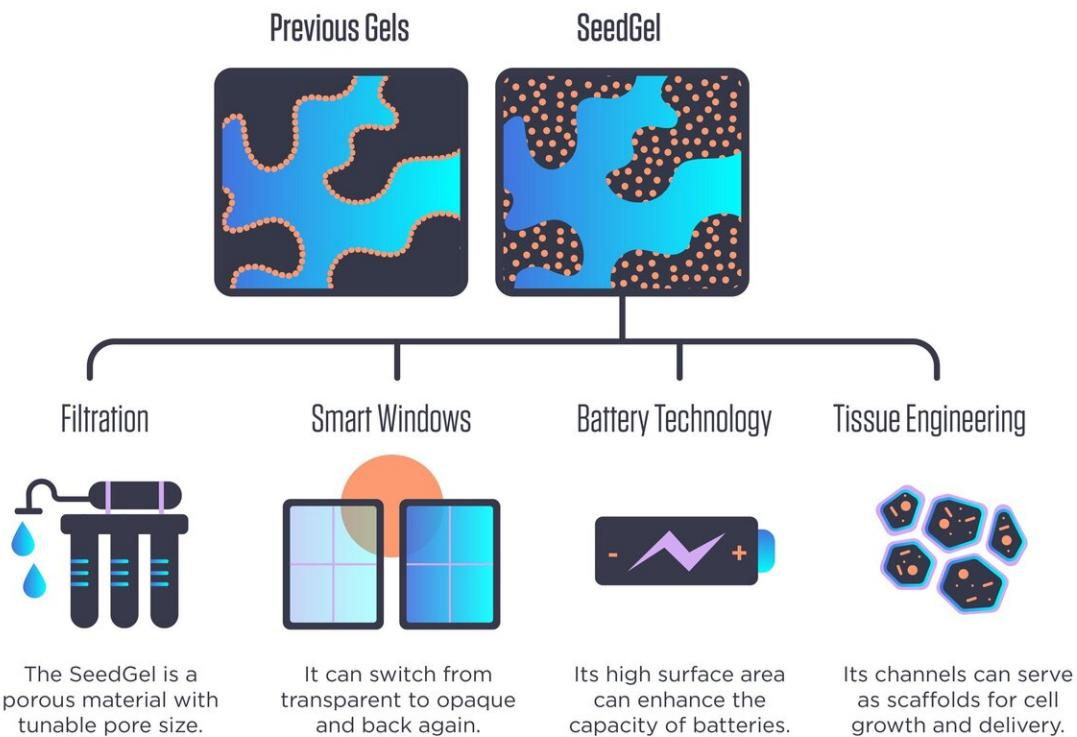
Unlike other gel-creation approaches, where nanoparticles remain at the interface between the gel's two constituent solvents (top left), the new approach concentrates nanoparticles in the interior of one of the solvents (top right), giving the resulting "SeedGel" unusual mechanical strength. The method could lead to gels that could be manufactured at industrial scales for a wide variety of potential applications. Credit: N. Hanacek / NIST
