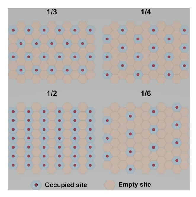
Occupation patterns for various electron occupancy levels in the moiré lattice. Credit: Microwave Nano-Electronics Lab, UC Riverside.
