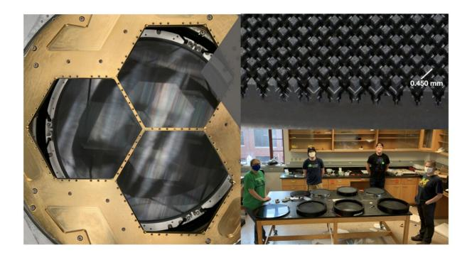
Left: One of the lenses developed by McMahon's team is installed in a camera assembly. Top right: This shows a close-up view of the stepped pyramid metamaterial structure responsible for the lens' antireflective properties. Bottom right: Members of the McMahon lab stand by recently fabricated silicon lenses. Credit: Jeff McMahon
