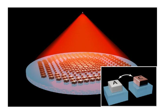
A new MIT-fabricated metalens shifts focus without tilting, shifting, or otherwise moving. The design may enable miniature zoom lenses for drones, cellphones, or night-vision goggles. Credit: Massachusetts Institute of Technology
