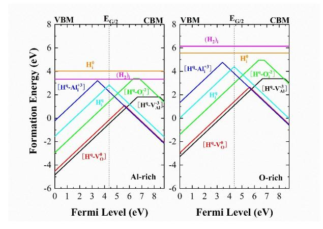
Formation energies of H-defect complexes in irradiated  $\alpha$ -Al2O3 as a function of the Fermi level in Al-rich (left) and O-rich (right) growth environments. Credit: PAN Xindong
