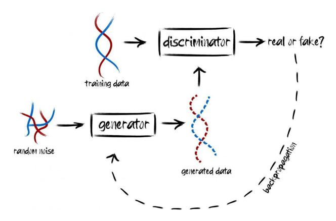
A generator machine shapes random noise while a discriminator machine tests the generated data against a database of available real data. Once the process is complete, the algorithm will generate artificial data that looks like the real one, but is actually completely new. Credit: Yelmen et al. 2021
