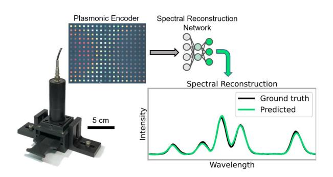
Neural network-based on-chip spectroscopy using a scalable plasmonic encoder. Credit: UCLA Engineering Institute for Technology Advancement
