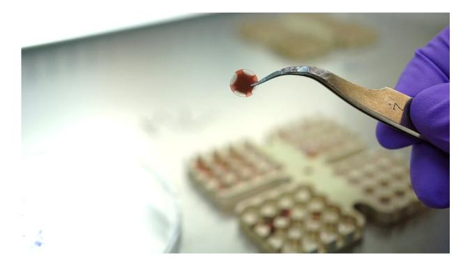
Quartz disc with dried Aspergillus niger spores, before being placed in the aluminum sample carriers that went on the Trex-box Credit: German Aerospace Center (DLR)
