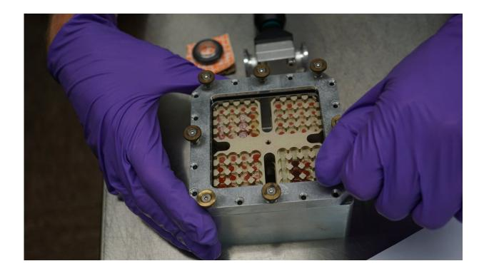
Trex-box being sealed after sample preparation at DLR. You can see the top layer harboring the quartz disc that carry the dried microbial samples Credit: German Aerospace Center (DLR)
