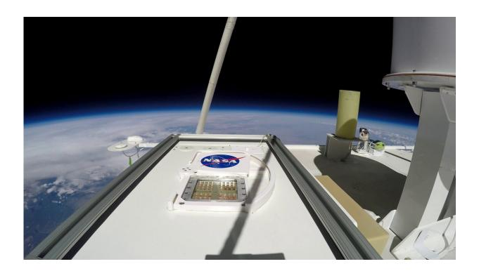
MARSBOx payload in the Earth's middle stratosphere (38 km altitude). The shutter is open exposing the top layer samples to UV radiation. Credit: NASA
