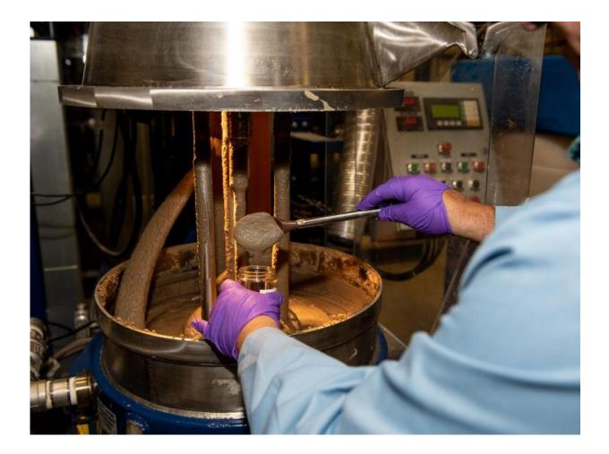
PNNL researchers are exploring how to cost-effectively turn mush like this into biofuel. As part of their efforts to scale up production and gain the efficiencies needed for wide-scale adoption, they have tested a variety of potential feedstocks including spent grain from a local brewery, shown here, as well as cafeteria wastes and kitchen scraps. Credit: Andrea Starr | Pacific Northwest National Laboratory
