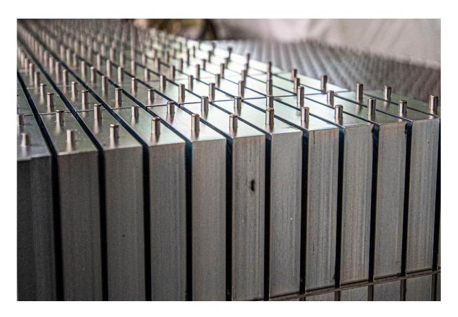
An array of 520 calorimeter towers, each consisting of 36 steel absorber blocks interleaved with scintillator tiles and the pins that hold them together. Credit: Brookhaven National Laboratory
