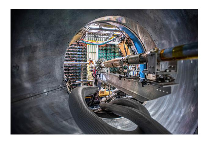
A view through the STAR endcap magnet at the new calorimeter components installed in the "forward" direction. These components will allow physicists to measure and reconstruct the energy of jets from particles emerging close to the beamline. Credit: Brookhaven National Laboratory
