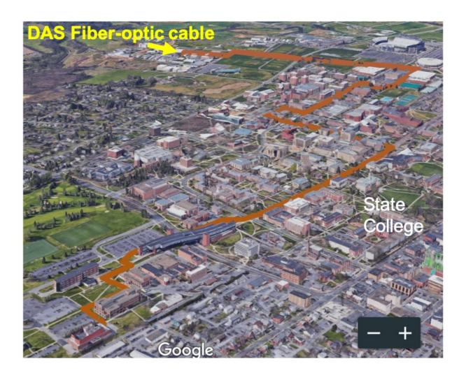
Bird's-eye view of the fiber-optic cables used for the FORESEE project in which scientists used pre-existing cables to monitor geological events. Credit: Foresee, Penn State
