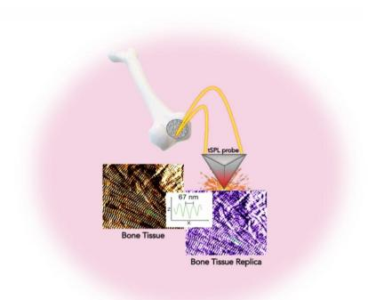
Researchers were able to replicate — with sub-15 nm resolution — bone tissue structure in a biocompatible material using thermal scanning probe lithography. This method opens up unprecedented possibilities for pioneering new stem cell studies and biomedical applications. Credit: NYU Tandon School of Engineering
