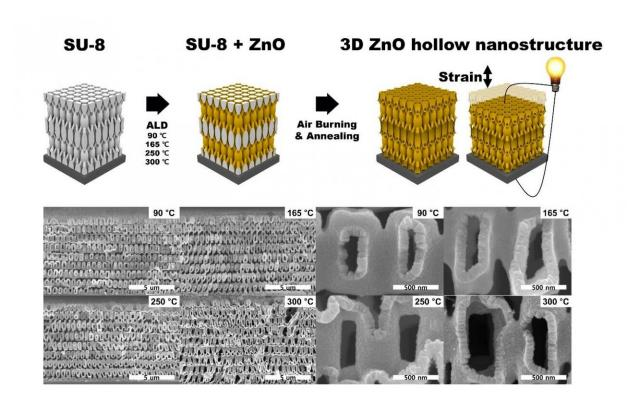
Conceptual schematics and SEM images of 3D ZnO hollow nanostructure deposited at 90, 165, 250, and 300 °C after removal of the epoxy template. Credit: KAIST
