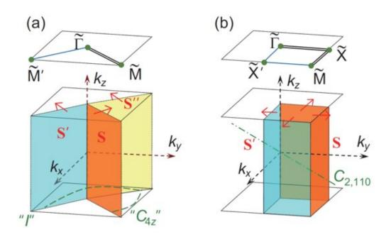
The definition of  $\chi$  in systems with S4 symmetry on the orange surface S. The system in (b) has C2,110 symmetry. Credit: Science China Press
