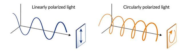
Laser light is usually linearly polarized, meaning that its waves oscillate in only one direction - up and down, in the example at left. But it can also be circularly polarized, at right, so its waves spiral like a corkscrew around the direction the light is traveling. A new study from SLAC National Accelerator Laboratory and Stanford University predicts that this circularly polarized light can be used to
