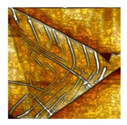
The base of the 2D-material with the white lines showing the structural kinks which modify the electrical properties mechanically. Credit: University of Sussex
