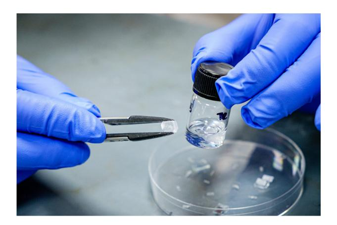
A close up of the new piezoelectric crystal developed by NTU scientists, which can flex up to 40 times more than the conventional ferroelectric crystals typically used in small actuators and sensors.
