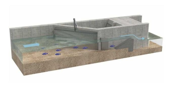
A safe guidance system for fish: a specially designed bar rack effectively guides downward migrating fish past the turbine, only slightly limiting the power plant's operations. Credit: VAW / ETH Zürich
