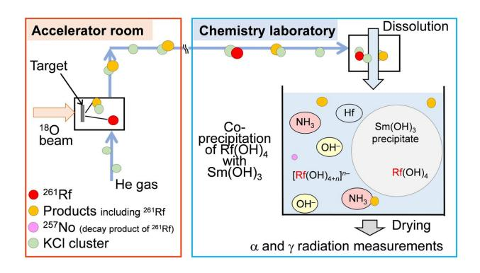
Fig.2 Schematic diagram of online co-precipitation experiment of <sup>261</sup>Rf. (credit: Osaka University
