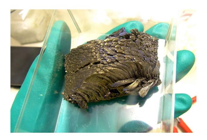
The chemical element Europium, ~300g ingot, crystalline sublimed dendritic, high pure 99.998% Eu/TREM (TREM = Total Rare Earth Metal). Handled in a glovebox under the inert gas argon. Credit: Alchemist-hp (pse-mendelejew.de) CC0 public domain
