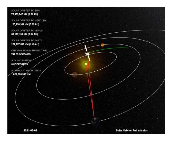
A visualisation showing how the trajectory of Solar Orbiter takes it within 5° of the Sun, as seen from Earth (indicated with red lines). This marks the start of Solar conjunction, lasting from about 29 January until about 14 February 2021. In the image, the Sun is shown much, much smaller than it should be so as to not cover up the spacecraft. Earth is the dark blue orb in the foreground. Credit: ESA
