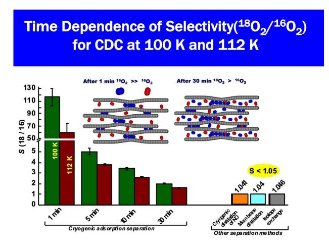
Comparison of S at different times at 100°K and 112°K for the CDC in this work with other separation methods from the literature. The inset shows illustrative models for the pore filling of CDC by  $O_2$ -16 and  $O_2$ -18 molecules after 1 min and 30 min. Credit: Copyright 2021, *Nature Communications*,
