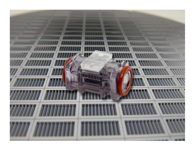
The electrodes for the ozone generator are made of silicon wafers with precisely etched trenches. Credit: Fraunhofer-Gesellschaft
