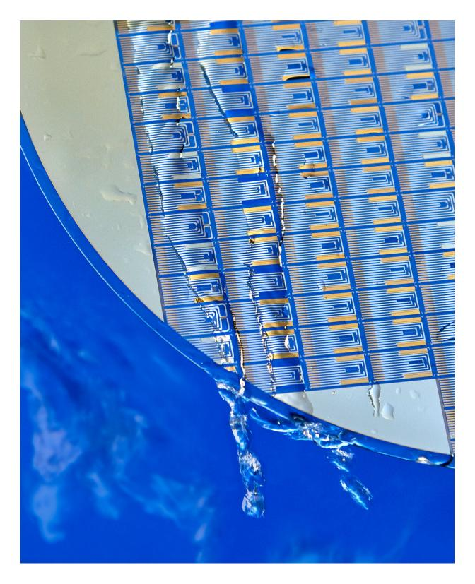
The Fraunhofer ISIT sensors are incorporated in glass wafers. Credit: Fraunhofer-Gesellschaft
