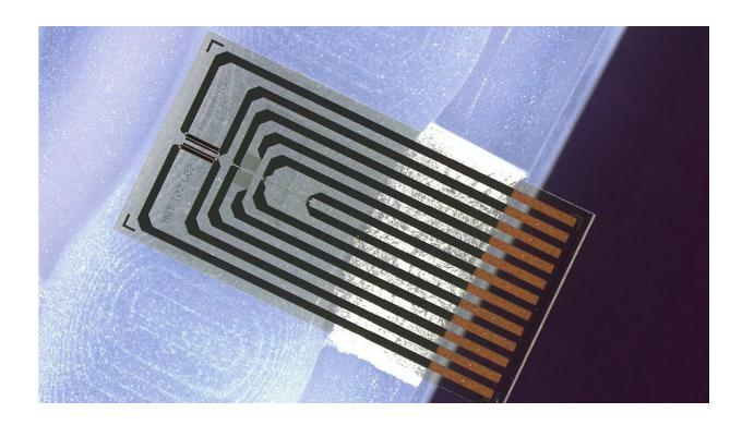
Sensors measure mass flow, temperature and conductivity. Credit: Fraunhofer-Gesellschaft
