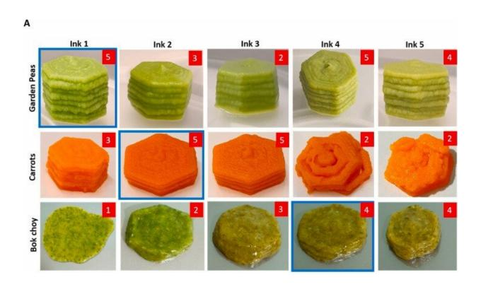
Representative images of 3D printed shapes with five formulations of one food ink type, images with box drawn around them represent the optimised formulations of the inks. Print scores represented on top right corner assessed by shape fidelity and shape stability. Credit: SUTD / NTU / KTPH
