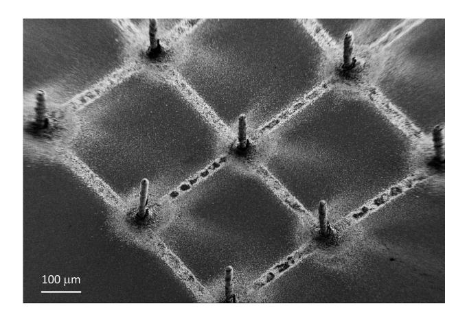
Example of the deposited perovskite pillars, defining a pixel for the creation of an image. Credit: L. Forró, EPFL.
