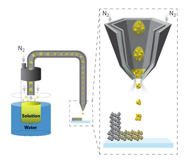
Schematic representation of the Aerosol Jet Printing method developed in this study. The agitated methylammonium lead iodide perovskite solution is focused to a predefined position at the nozzle by the nitrogen (N2). The particularity of the material is that formed nanocrystals in flight do not spread out on the graphene substrate, allowing the creation of 3D architectures. Credit: Glushkova et al *ACS Nano*.
