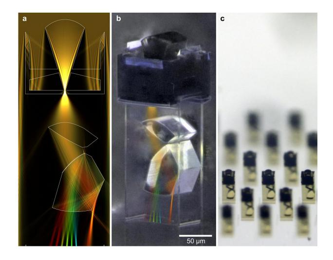
3D-printed miniature spectrometer. a, wave-optical simulation of the spectrometer. b, microscope image of the fabricated spectrometer overlayed with the intensity distribution from a. c, array of fabricated spectrometers. Credit: Andrea Toulouse, Johannes Drozella, Simon Thiele, Harald Giessen, and Alois Herkommer
