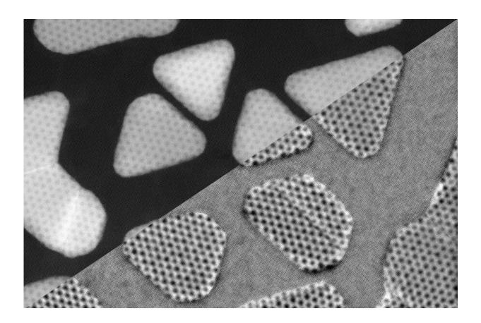
Caption:These images of "islands" of gold atoms deposited on a layer of twodimensional molybdenum sulfide were produced by two different modes, using a new scanning tunneling electron microscope (STEM) in the new MIT.nano facility. By combining the data from the two different modes the researchers were able to figure out the three-dimensional arrangement of atoms where the two materials meet. Credit: Massachusetts Institute of Technology
