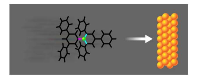
A Reichardt's dye molecule colliding at hyperthermal velocity with a copper surface. The molecule's orientation determines whether the energy of the collision is concentrated in one of the bonds between the central nitrogen atom (green) and a carbon atom in one of the surrounding rings (black). Credit: L. Krumbein et al. ; adapted by APS/Alan Stonebraker
