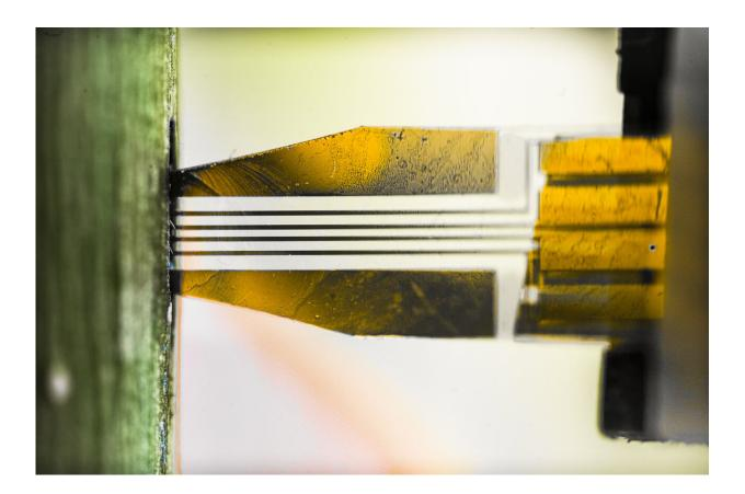
An implantable organic electrochemical transistor sensor. Credit: Thor Balkhed
