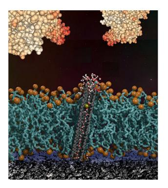
A cross section of a lipid bilayer with a carbon nanotube pore on a surface of a bioelectronic device. The bilayer protects the surface from large protein foulants in solution and lets water, ions, and small molecules through to the device surface. Credit: Yuliang Zhang and Aleksandr Noy (LLNL)
