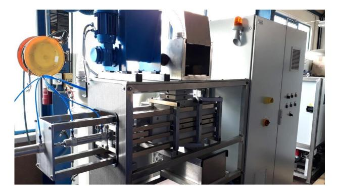
A demonstration plant for the regeneration of the activated carbon. Credit: Fraunhofer-Gesellschaft
