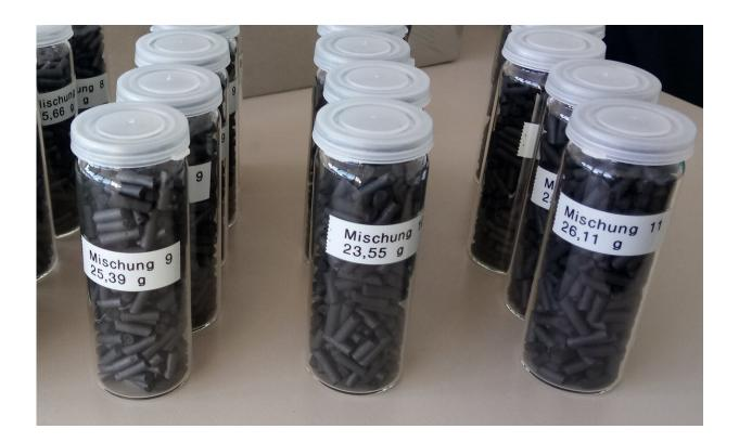
The activated carbon composite from Fraunhofer has an electrical conductivity three times that of conventional granular activated carbon. Credit: Fraunhofer-Gesellschaft
