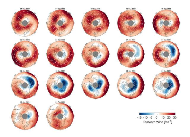
Based on data from ESA's Aeolus wind mission, the image shows how the polar vortex in the lower stratosphere changed between 1 December 2020 and 1 February 2021. The first few plots at the beginning of December show the vortex in a comparatively normal state, but in mid-December patches of blue wind appear, and the wind is going backwards relative to normal conditions. Credit: University of Bath/C. Wright
