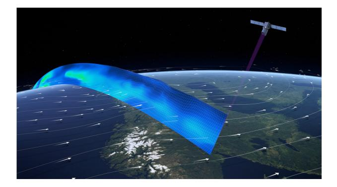
The Aeolus mission was not only built to advance our understanding of atmospheric dynamics, but also to provide much-needed information to improve weather forecasts. The satellite carries the first wind lidar in space, which can probe the lowermost 30 km of the atmosphere to provide profiles of wind,
