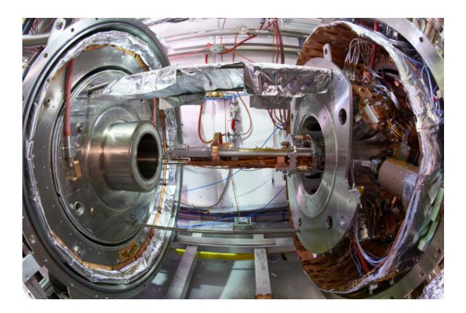
The AEgIS experiment is built around two powerful superconducting solenoids. Credit: CERN
