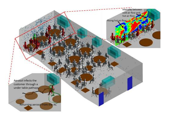
In *Physics of Fluids*, researchers report using advanced simulation methods to capture the complex flows that occur when the cold airflow from air conditioners interacts with the hot plume from a dining table and the transport of virus-loading particles within such flows. Schematic of the flow and particle transport, highlighting the two transport pathways, within the entire restaurant. Mannequins show where customers were seated. Credit: Han Liu
