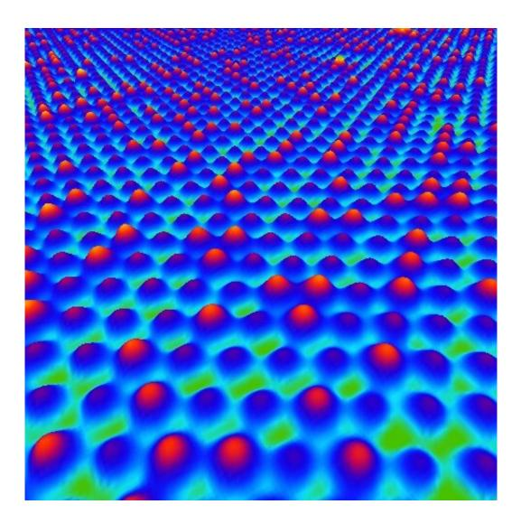
Close-up of the semiconducting 2D alloy. Scanning tunneling microscopy image of a Si-Ge alloy with a composition of Si5.67Ge0.33. Tall protrusions correspond to Ge atoms and short ones to Si atoms. The distance between protrusions is only 0.64 nm. Credit: Antoine Fleurence, JAIST
