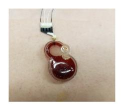
A small and inexpensive sensor, announced in Applied Physics Letters and based on an electrochemical system, could potentially be worn continuously by cardiac patients or others who require constant monitoring.Right: Wearable sensor attached to a patient's chest. Left top: Heartbeat signal acquired from the sensor. Left bottom: Acquired breathing signal. Credit: Yong Xu
