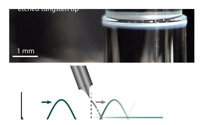
Top: An optical microresonator and a sharp tungsten tip. The tip's position can control the amount of back reflections in the microresonator. The authors show
