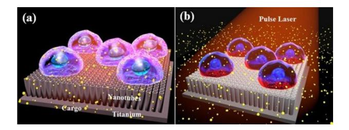
Pictorial representation of (a) cells cultured on top of titanium oxide nanotubes and (b) massively parallel photoporation using the interaction between an array of nanotubes and a pulse laser. Credit: Toyohashi University of Technology.
