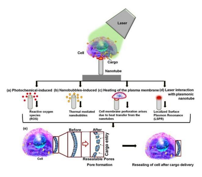
Schematic representation of possible mechanism of photoporation on titanium oxide nanotubes for cargo delivery. Credit: Toyohashi University of Technology.
