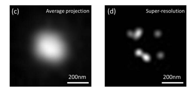
The image on the left (C) shows diffraction-limited imaging that is too blurry to capture plasmonic hotspots required to conduct single-molecule SERS analysis. On the right (D) is super-resolution imaging of the same plasmonic hotspots using DNA-STROBE, which is clear enough to allow for single-molecule SERS analysis. Credit: Johns Hopkins University
