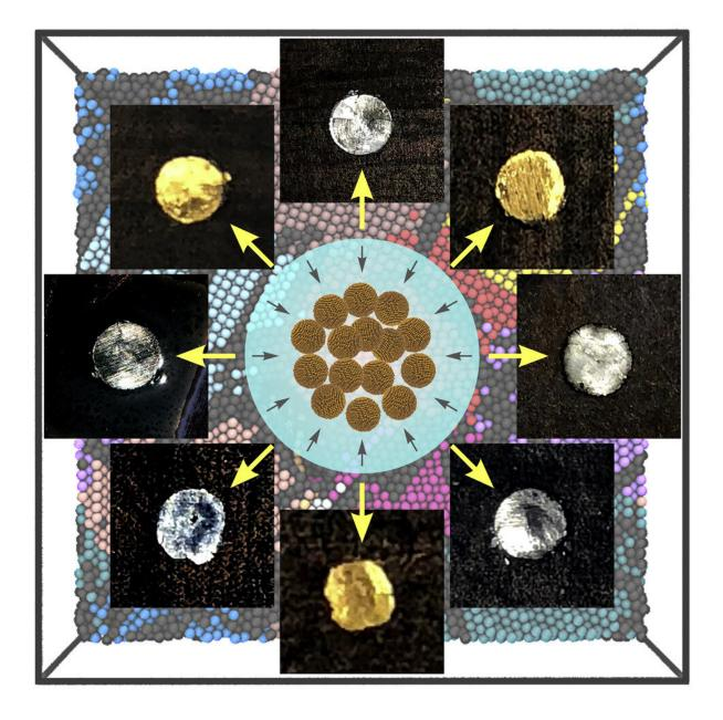
Researchers from Brown University have demonstrated a way to make bulk metals from nanoparticle building blocks. For a new study, the team made metal "coins" from nanoparticles of gold, silver, palladium and other metals . Credit: Chen lab / Brown University
