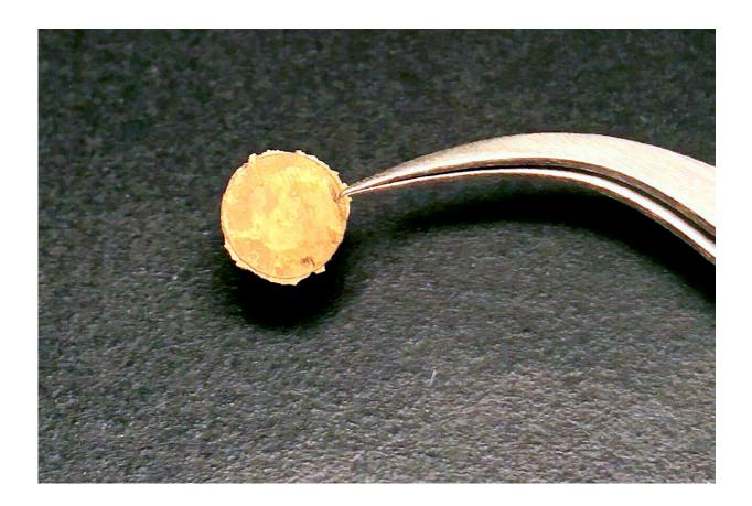
This gold "coin" was made from nanoparticle building blocks, thanks to a new technique developed by Brown University researchers. Making bulk metals this way allows for precise of the metal's microstructure, which enhances its mechanical properties. Credit: Chen Lab / Brown University
