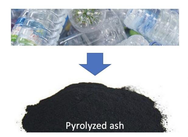
Rice University chemists turned otherwise-worthless pyrolyzed ash from plastic recycling into graphene through a Joule heating process. The graphene could be used to strengthen concrete and toughen plastics used in medicine, energy and packaging applications. Credit: Tour Group/Rice University
