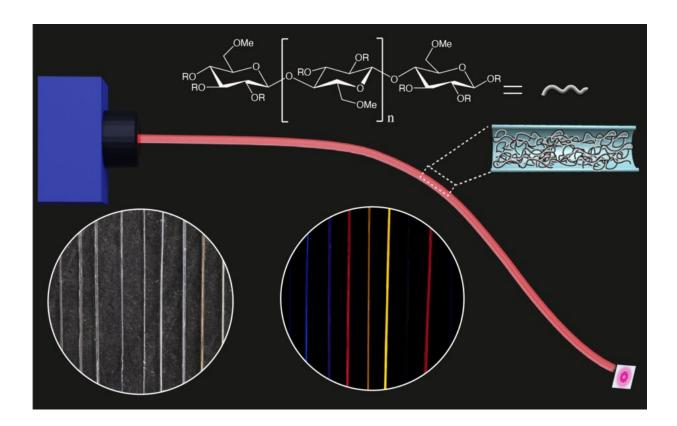
Schematic illustration of a light coupled optical fibre and photographs of methylcellulose-based optical fibers under ambient light and UV light. Credit: Ville Hynninen and Nonappa
